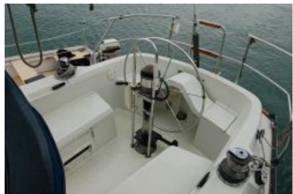
PRIMARIES PLACED AFT
